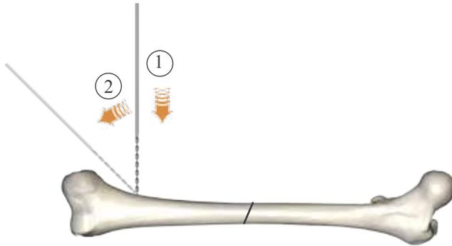
Fig. 2: Option 2 - Vertical „predrilling“ with drill bit (1), then turn in axial direction (2)
