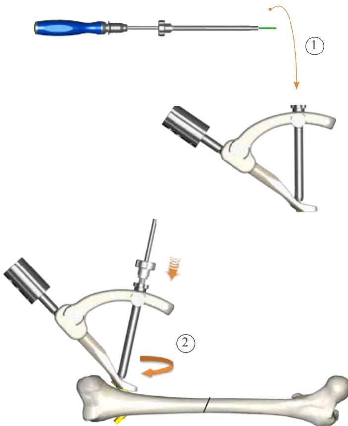
Fig. 13: Fixation of first plug by means of screw
